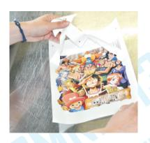
**6)** Heat-press the material at 145°C for 12 seconds, wait 5 seconds and remove the support. We suggest to re-heat press the material for another 5 seconds, protecting the print with a silicon paper.
