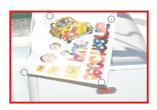
**4)** After cutting, peel the excess material by holding the hand resting on the support and do a little pressure to the outside.
